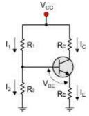
Given  $R_1$ =20K,  $R_2$ =10K,  $R_C$ =4K,  $R_E$ =5K and  $V_{cc}$ =30V
